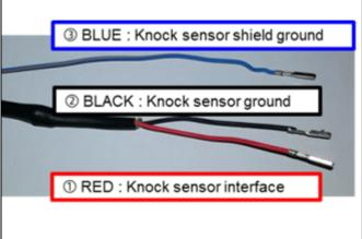
11. Cut off and discard the (3) original terminals from the ECM connector and fold the original wires (K) back onto the original engine control wire harness and secure with tape. Secure any excess wire from the new wire harness extension onto the original engine control wire harness with tape.
