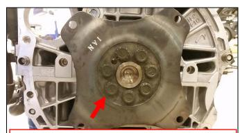
Install new drive plate/flywheel bolts (ONLY if new bolts are included with the replacement engine)
